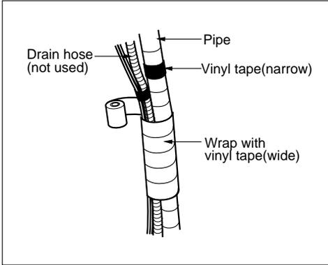
Do pipe forming by wrapping the connecting cable and refrigerant pipe (between the indoor unit and outdoor unit) with thermal insulation material and secure it with two kinds of vinyl tape.
