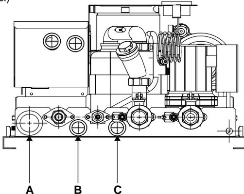
Hole A, B : for AC line (wire which is connected to the terminal block of the control box)
